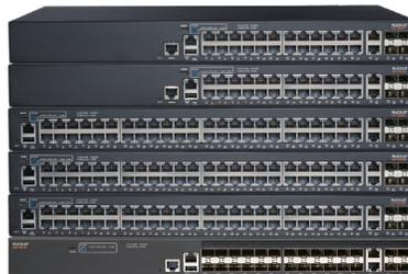
The standard Ruckus ICX 7150 switches are available in 24-, and 48-port 10/100/1000 Mbps models with four 1/10 GbE dual-purpose uplink/stacking ports. These switches are available with or without PoE+ power. Silent operation is available for out-of-closet environments.
