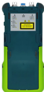
Modul FQ GLASFASER QUAD MULTIMODE 850/1300 nm SINGLEMODE 1310/1550 nm
