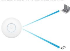
MU-MIMO with 3x3 and 1x1 clients: Each client radio of the the UniFi XG AP communicates with one 3x3 client and one 1x1 client at a time.
