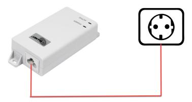
Connect the "LAN IN" port of the ALL0488v6 to the network/switch.
