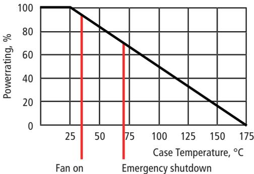
**Derating Using Case Temperature ( $T_c$ ):**
