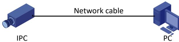
Use a Shielded Twisted Pair (STP) cable to connect the network interfaces of the network camera and the PC.
