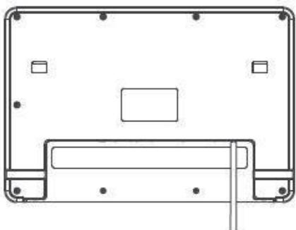
Plug the power cable into port of device
