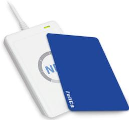
The ACR122 is a PC-linked Contactless Smart Card Reader/Writer developed on the 13.56MHz Contactless Technology. It is the world's first CCID Compliant Contactless Card Reader/Writer that follows both ISO14443 and ISO18092. This device is designed to support not only MiFare and ISO14443 Type A and B Cards but also FeliCa and NFC tags.
