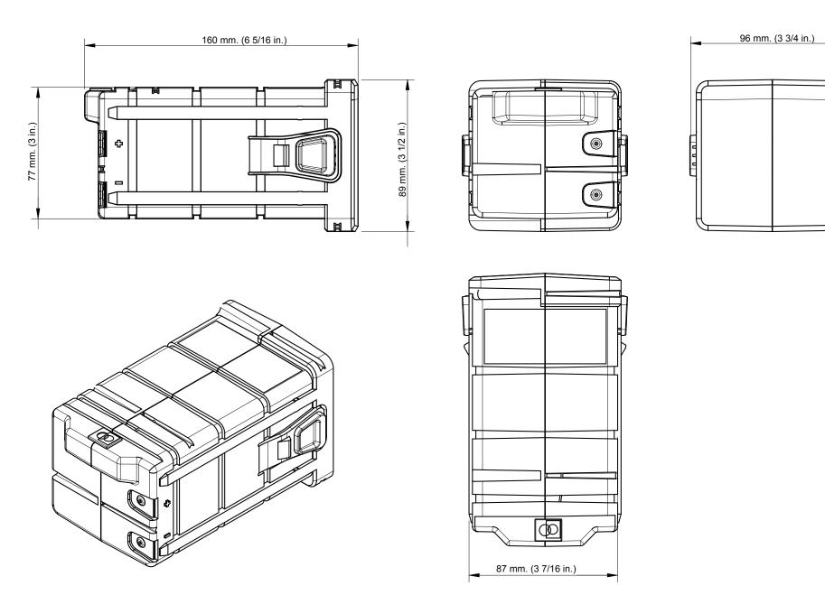
AXIS Installation Tool Battery 12V 3.4 Ah AXIS 12 JUNE, 2015 Scale 1:2
