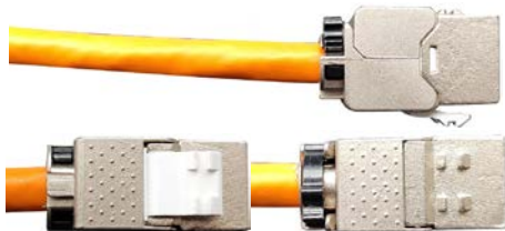
⑩.Fasten smart cable ties for 360 degree shielding
