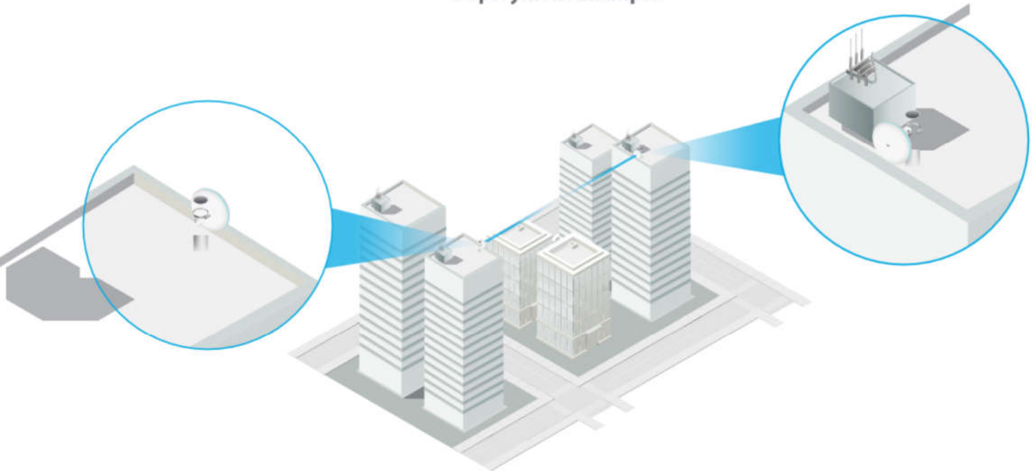
The UBB creates a wireless link between two buildings.
