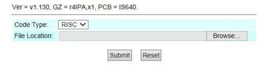
Step 2: enter [select file] interface, to select [gz] file to be updated [for example, VP5110\_70105.gz], and then press [open] (as shown in the following picture), to return to the main interface.
