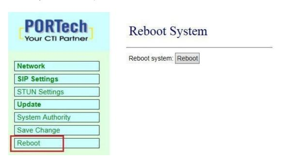
Step 1: click [Reboot] in the main interface to enter [Reboot System] and then press [Reboot] to reboot the system (as shown in the following picture).
