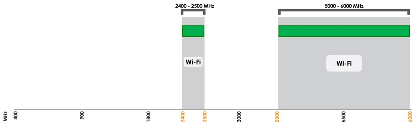
Indicates the Wi-Fi bands on which HELI-40 works
