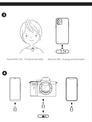
The receiver adopts a replaceable interface design. Three types of connectors
