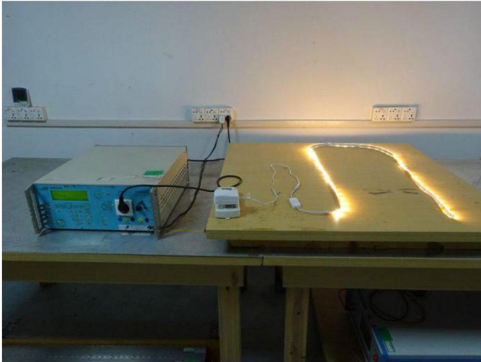
Surge ,EFT,Dip Test Setup
